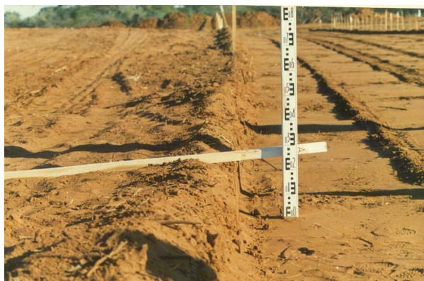
Photo 4-5 – Collapse settlement of sand subgrade: In excess of 150 mm was obtained along a section of the Serowe-Orapa road in Botswana after compaction to near refusal by a 25 kJ high energy impact compactor.
