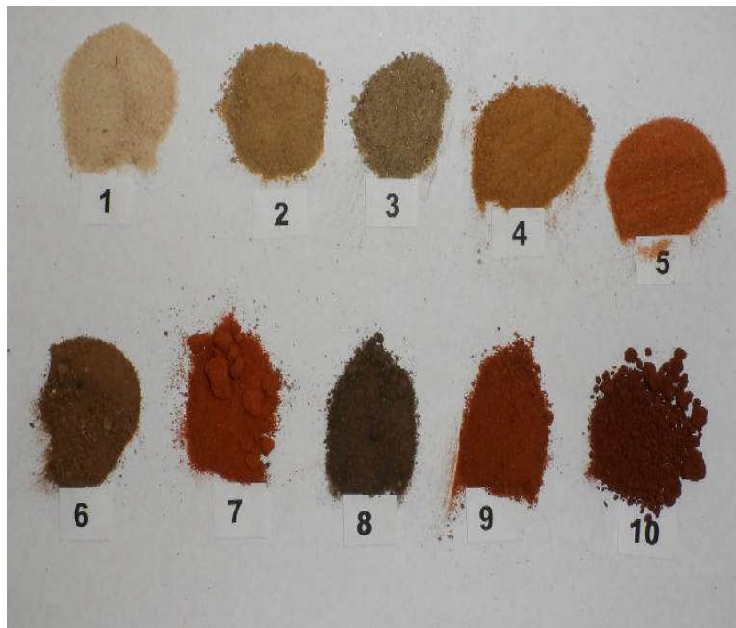
Photo 4-1: Colour scale used for ranking of sands by darkness
