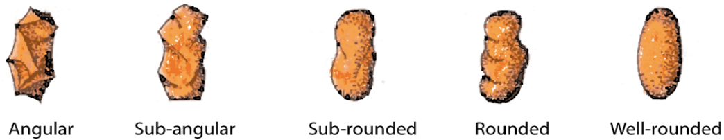
Figure 4-13: Degree of particle roundness
