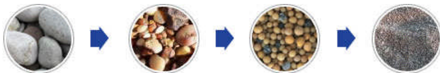
Figure 2-1: Formation of sand by erosion and weathering of rocks
