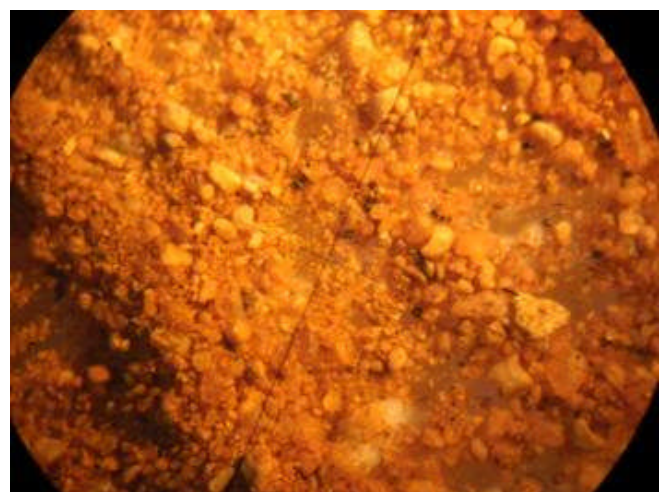
Photo 4-3: Example of poorly sorted, angular to sub-rounded sand (circled particle = 1 mm in dia.)
